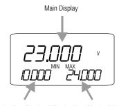
Auxiliary Display, MIN Auxiliary Display, MAX
