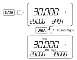
If the next measured value stored to memory deviates from the first by less than 0.33% of the measuring range, two acoustic signals are generated (DATA Compare).
